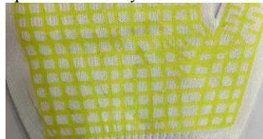
Figure 2. PET-G 3D-printed overlay structures applied on PES using (A) contact welding and (B) ultrasonic welding.
