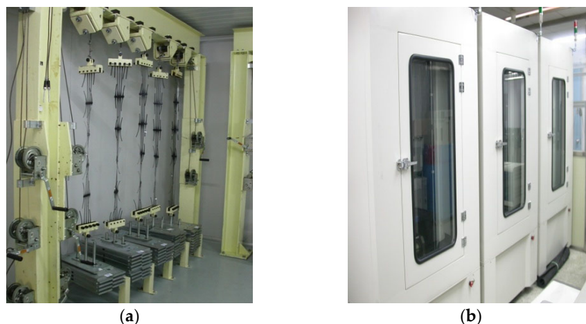
Figure 2. Photographic images showing the equipment employed to perform the (a) conventional creep and (b) SIM tests for the HDPE geogrids.
