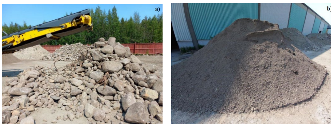
Figure 1. (a) Sorted coarse fraction from test box, (b) Sorted fine fraction from test box 2. A total of approx. 100 tonnes of contaminated fine fractions were obtained during the sorting process.
