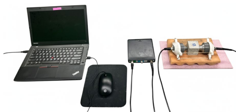
Figure 1. Computer with data acquisition system, oscilloscope, and the specimen with ultrasonic transducers used in present study to measure nonlinear ultrasonic parameters for concrete cube specimens.
