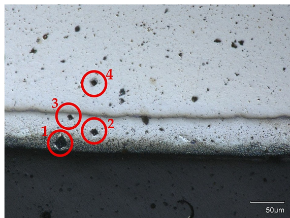
Figure 9. Example of hardness measurements indication position for sample 2. Number of indentations acc. to Table 5.
