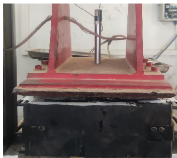
(a) Compaction process
