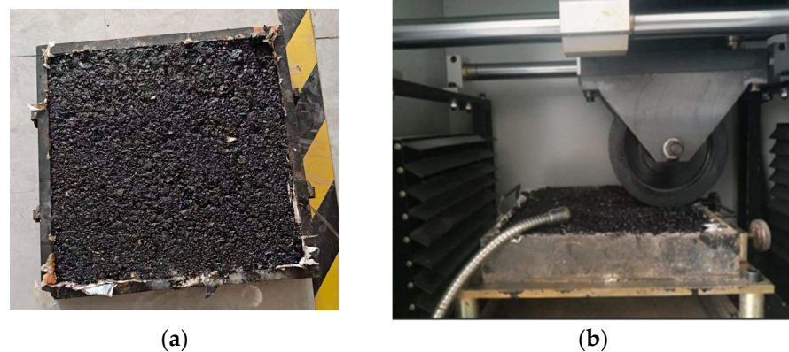
Figure 4. Rutting Test of Fiber-Reinforced Asphalt Mixtures: (a) Asphalt Mixture Rutting Slab. (b) Rutting Test Procedure.
