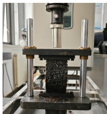
Figure 7. Splitting Test of Fiber-Reinforced Asphalt Mixtures.
