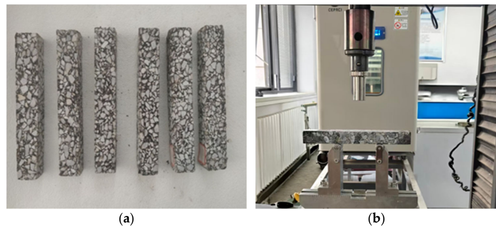
Figure 5. Beam Specimens of Fiber-Reinforced Asphalt Mixtures: (a) Beam Specimens of Asphalt Mixtures. (b) Low-Temperature Crack Resistance Test.
