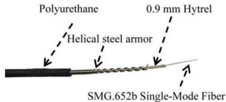
Figure 2. Armored Bragg fiber optic sensor [29].
