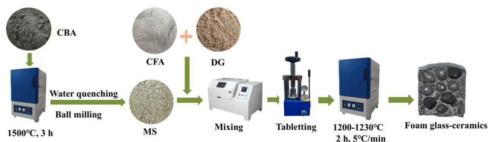
Figure 2. Preparation procedure of foam glass-ceramics.
