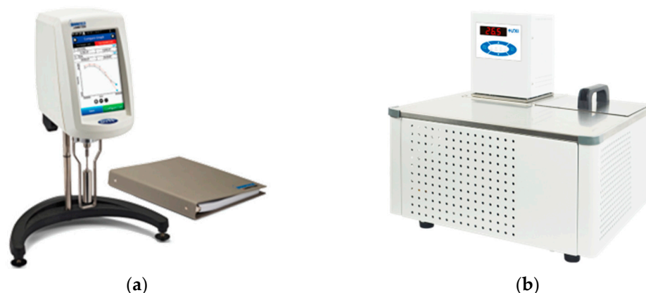
Figure 4. Experimental instrument: (a) rotational rheometer; (b) horizontal high- and low-temperature constant-temperature bath.
