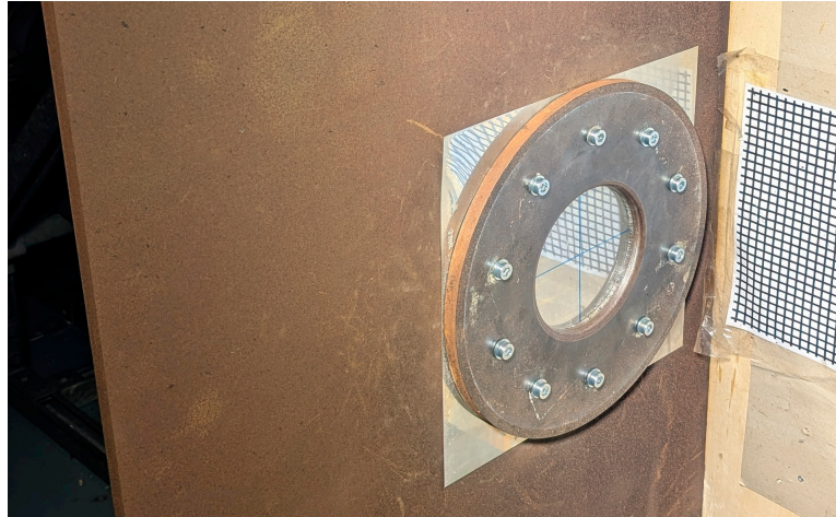
Figure 2. Detail of the clamped circular target plate. The annular fixture constrains the specimen around the exposed circular region. The rear surface remains visible to the high-speed camera and carries the reference marks used for video processing.
