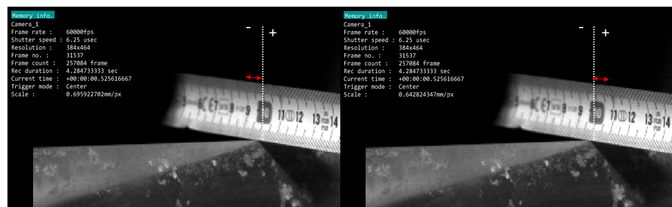
Figure 4. Perspective correction used in the proposed method. The apparent displacement of each tracked point is measured as a signed perpendicular pixel offset (red arrow) relative to the reference diameter and converted into millimeter by a calibrated rational one-dimensional mapping.
