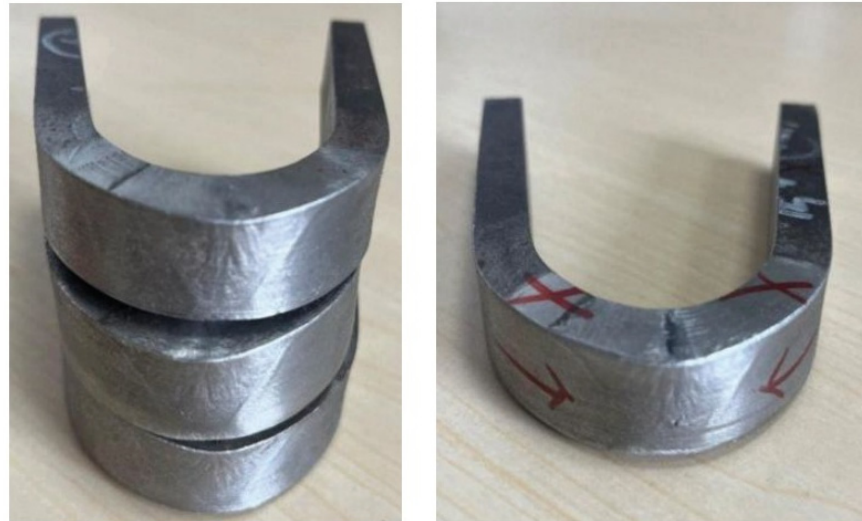
Figure 12. Welded joint side bend test specimens after 180° bending.
