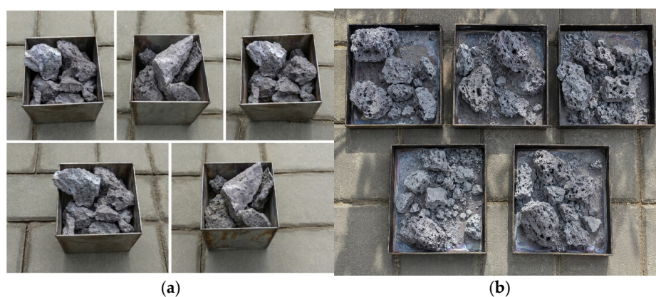
Figure 8. Experimental slag after testing with RDBO (a) and colemanite (b).
