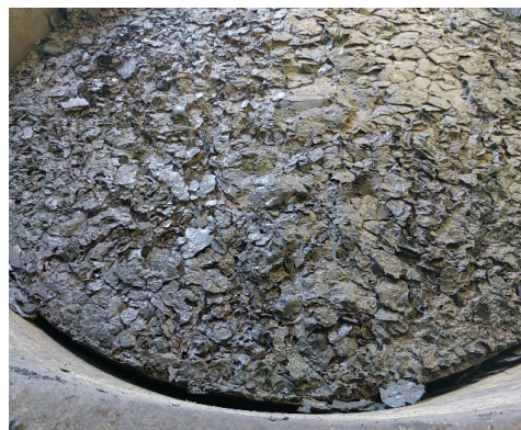
Figure 5. Slag after 168 h of holding in a slag pot under ambient conditions.
