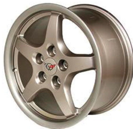
Figure 9. LPC magnesium alloy wheel for the Chevrolet Corvette [65].
