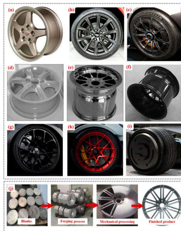
Figure 21. Development and application of magnesium alloy wheels [6]: (a) Chevrolet Corvette magnesium alloy wheel; (b) Cadillac CT4-V forged spin-formed magnesium alloy wheel; (c) AMG Project One biomimetic 9-spoke forged magnesium alloy wheel; (d) hollow billet extruded magnesium alloy wheel: (14 × 6) J; (e) hollow billet extruded magnesium alloy wheel: (13 × 6) J; (f) hollow billet extruded magnesium alloy wheel: (13 × 8) J; (g) Bugatti Chiron Super Sport 300+ Mg wheel; (h) Porsche
