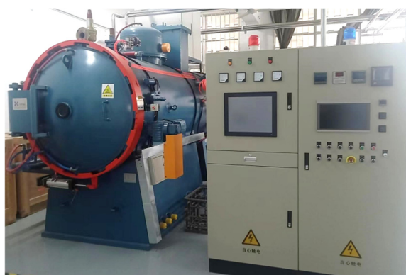
Figure 2. Experimental facility picture of double-chamber vacuum air-cooled oil quenching furnace.
