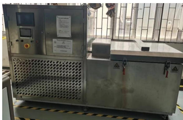
Figure 3. Experimental facility picture of liquid nitrogen hybrid deep freezer.
