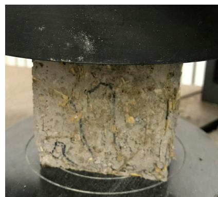
Figure 10. Compression failure of specimens in normal temperature.
