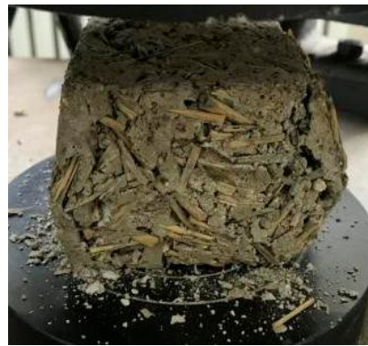
Figure 11. Compression failure of specimens after 15 times Freeze–Thaw Cycles.
