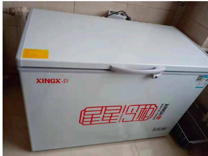
Figure 2. Test device of freeze-thaw cycles.
