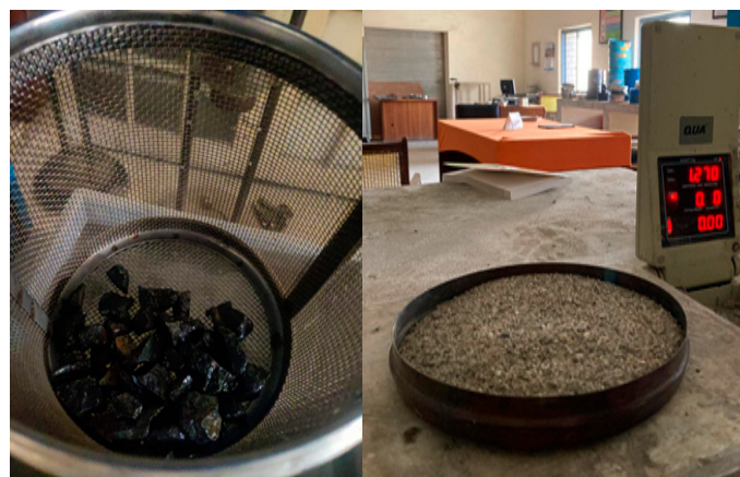
Figure 6. Laboratory testing of aggregates for physical characterization, including specific gravity determination and fineness modulus evaluation as per ASTM standards.
