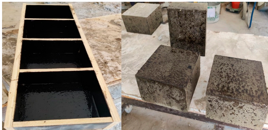
Figure 5. Preparation and casting of concrete shielding blocks using wooden moulds. The produced blocks were employed in radiation attenuation tests against Cesium-137 and Cobalt-60 gamma sources.
