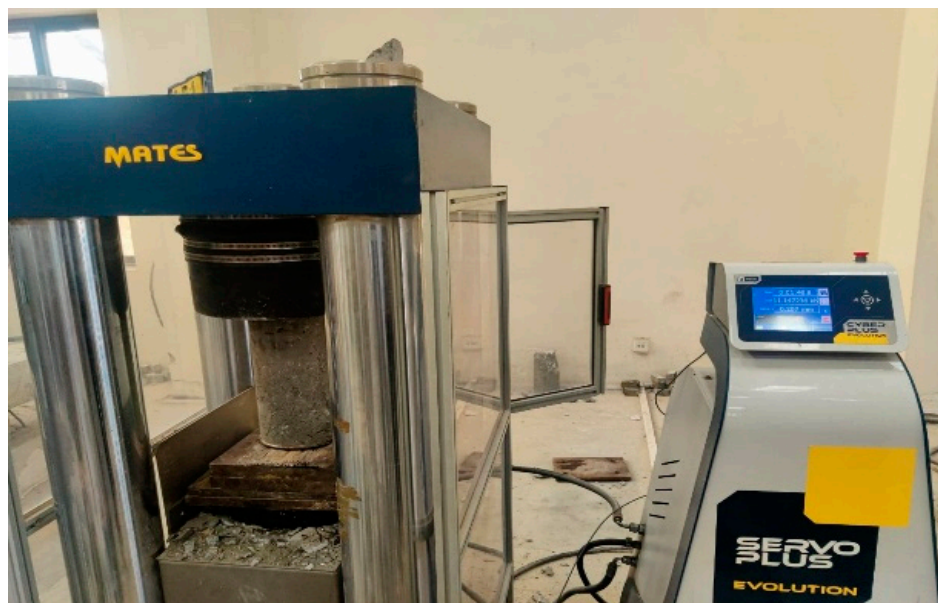
Figure 2. Compressive strength test setup for cylindrical concrete specimen conducted as per ASTM C39 standard using a universal testing machine (UTM).
