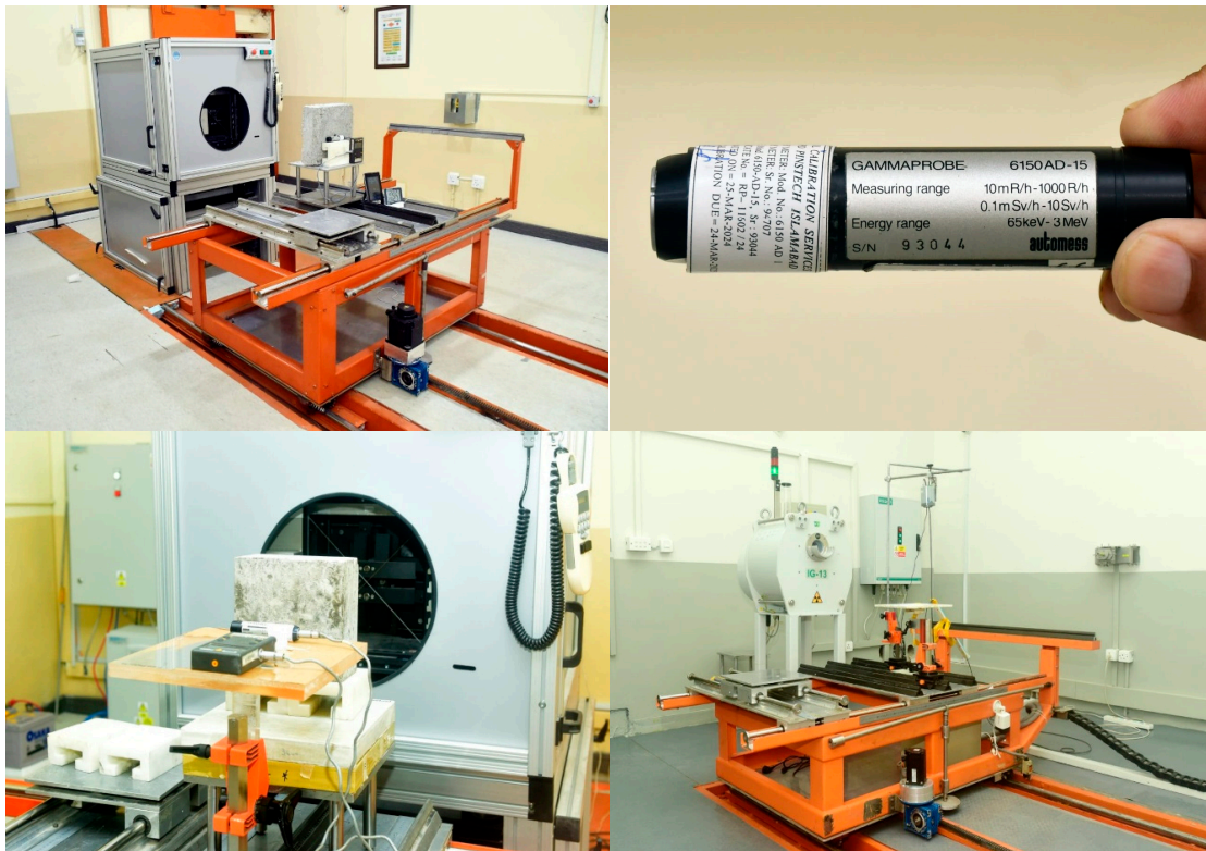
Figure 4. Experimental setup for the gamma radiation shielding test. The concrete specimen was positioned between the radioactive source (Cesium-137/Cobalt-60) and a gamma ray detector to measure transmitted radiation intensity and evaluate shielding effectiveness.
