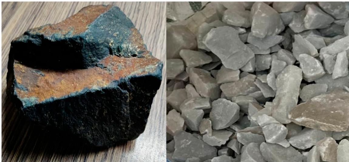
Figure 1. Magnetite (left) and dolomite (right) aggregates used as coarse aggregate materials in the experimental study.
