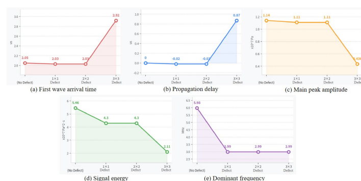
Figure 7. Comparison chart of ultrasonic signal characteristic parameters at different defect sizes of lateral monitoring points.
