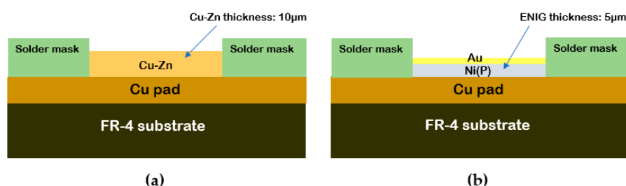
Figure 2. Schematic cross-sections of the two specimen types: (a) SAC305/electroplated Cu-20Zn, and (b) SAC305/ENIG. Layer thicknesses are indicated for each wetting layer configuration.
