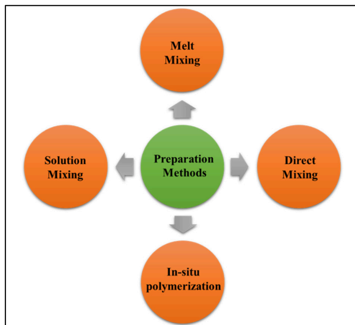
Figure 5. Different methods for preparation of MWCNT polyester nanocomposites.
