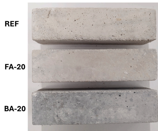
Figure 2. Hardened mortar prism specimens (REF, FA-20, and BA-20) used for mechanical testing.
