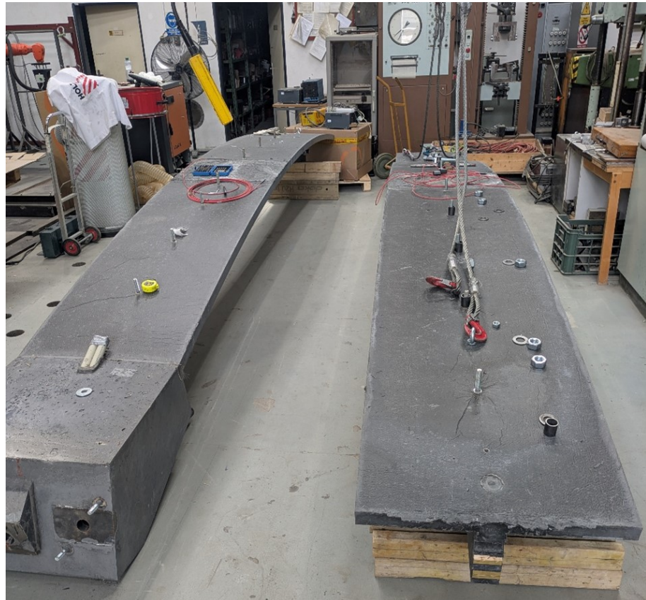
Figure 8. Assembly of two UHPFRC half-arch segments in mirror configuration prior to joint casting and post-tensioning.
