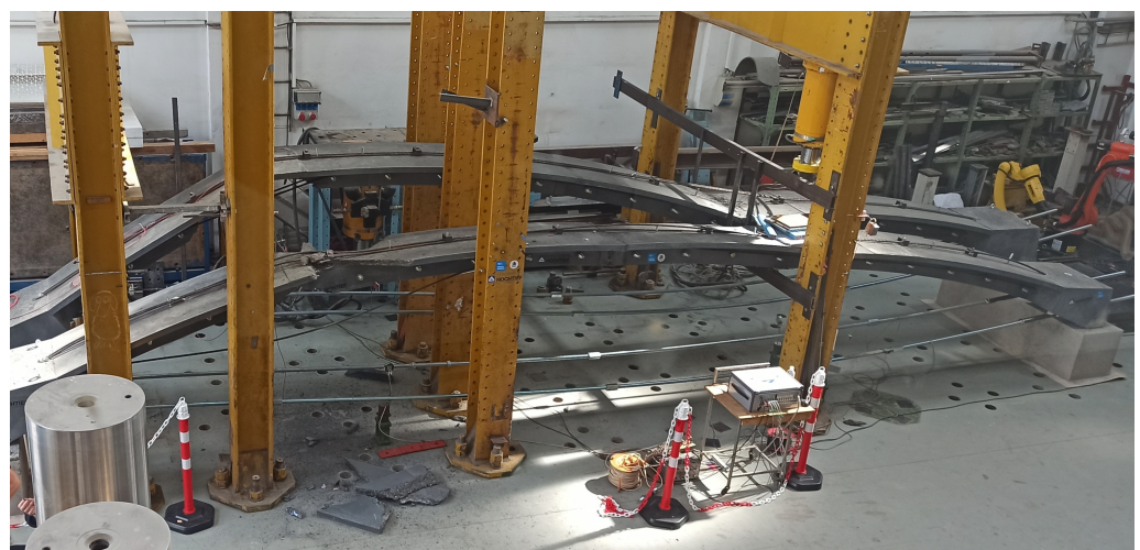
Figure 16. View of both broken arches.
