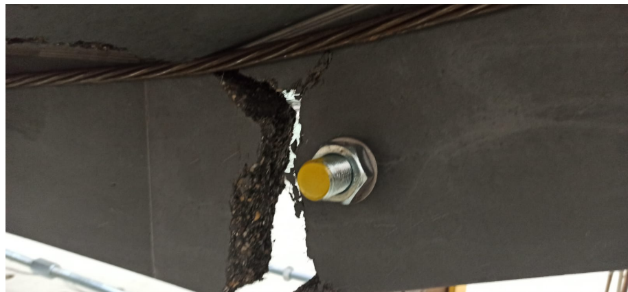
Figure 13. Experimental detail of first tensile crack.
