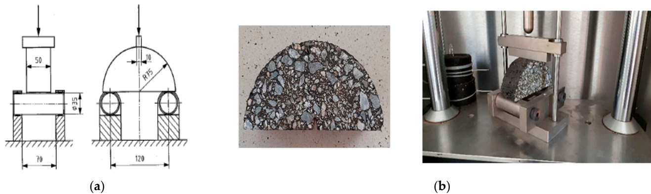
Figure 4. Test frame and SCB specimen: (a) schematic diagram (EN 12697-44) [63]; (b) SCB specimen during the test for the resistance to cracking (M.M. Iwański).
