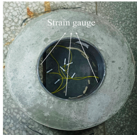
Figure 5. Mounting position of strain gauges.
