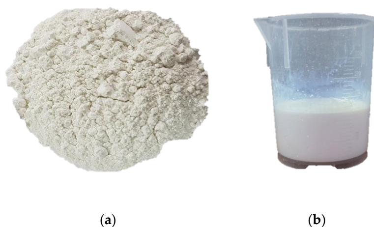
Figure 1. Materials used for the photocatalytic infiltration pavement block: (a) anatase TiO 2 powder and (b) SBR latex.
