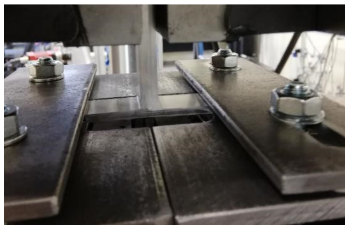
Figure 3. Specimen clamping arrangement in the dedicated fixture during the bending test.
