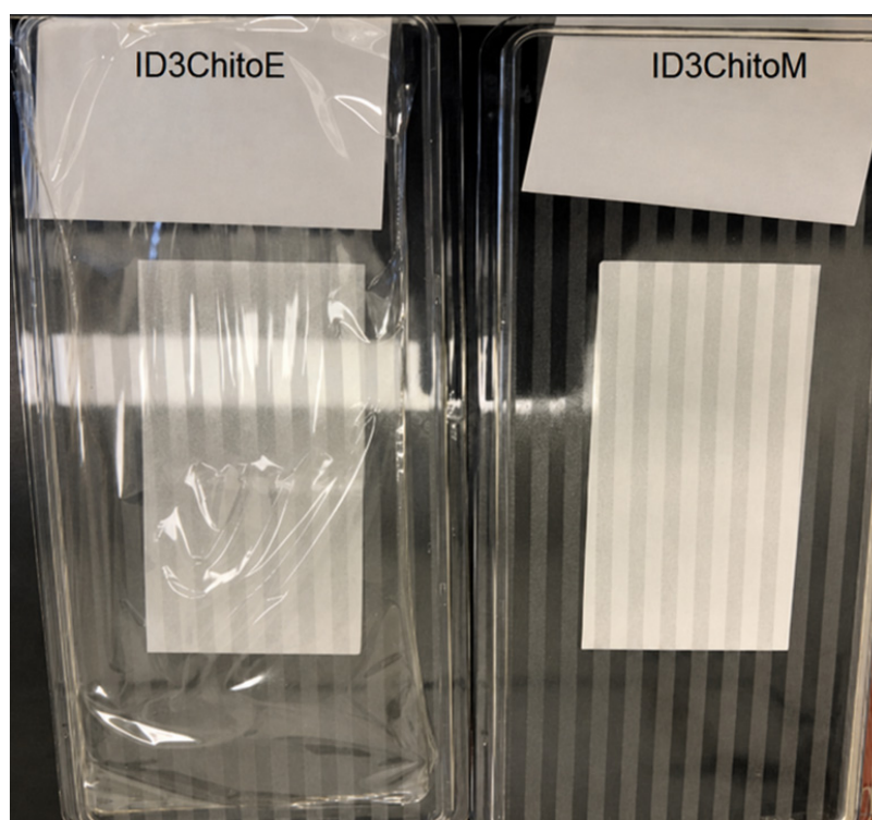
Figure 1. Chitosan films prepared from (AcOH, left) and (LA, right) solutions in PET plates.
