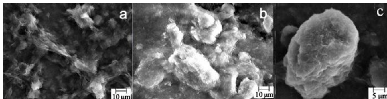
Figure 5. The SEM images of hectorite and OTMA + /hectorite: (a) hectorite; (b) and (c) OTMA + /hectorite.
