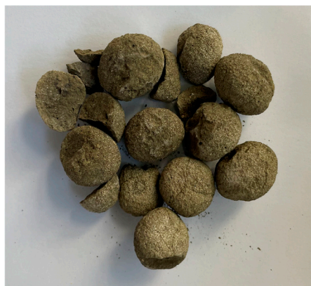
Figure 9. SWS clinker appearance at 1300 °C peak sintering temperature.
