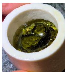
Figure 7. Amorphous product formed during Sintering 1 (sample type: reference; sample holder: ceramic crucible; peak temperature: 1450 °C).
