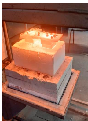
Figure 2. A drop-down oven base ensured rapid air cooling of the samples.
