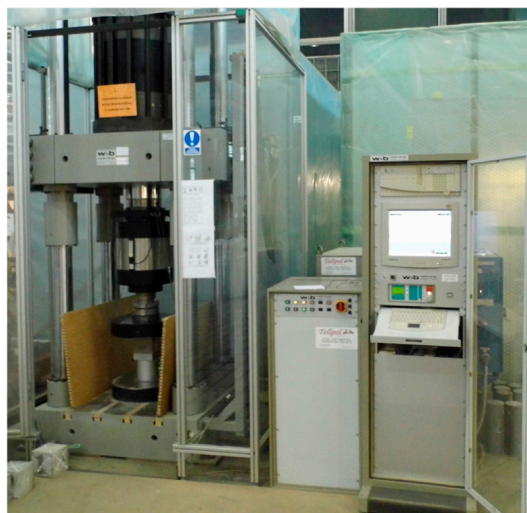
Figure 3. Walter+Bai a.g. strength testing machine used to test concrete compressive strength, tensile strength, and modulus of elasticity.
