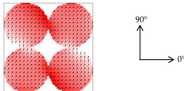
Figure 1. Sketch of the nanodot arrays under examination consisting of four touching nanodots (diameter 105 nm), embedded in air or in the other magnetic material, as well as orientation of the external magnetic field angles.
