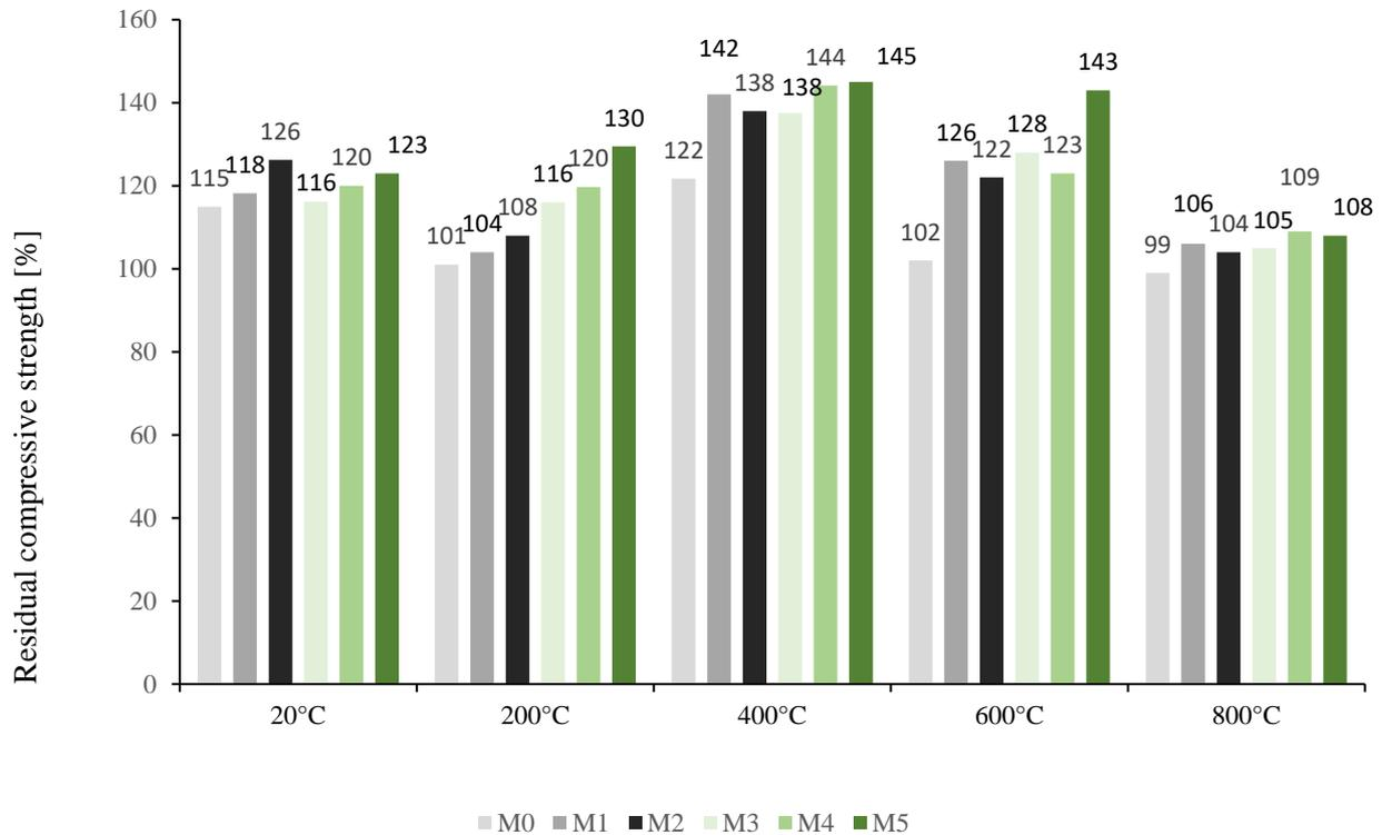
**Figure 4.** Relative compressive strength of the heated mortars after 24 months of further curing.
