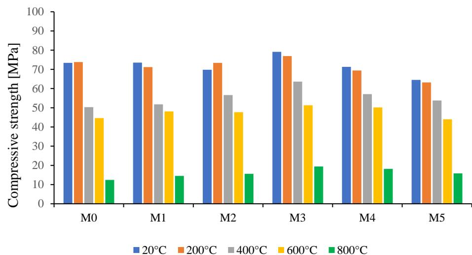
**Figure 2.** Compressive strength of the heated mortars.
