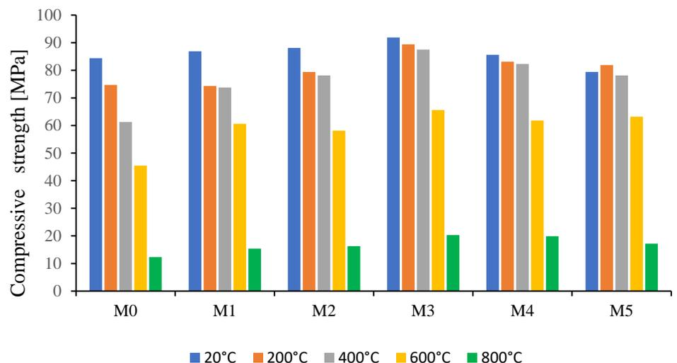
**Figure 3.** Compressive strength of the mortars after heating and curing for the next 24 months.
