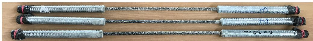
**Figure 1.** Specimens for tension tests ( $\text{Ø}12$  BFRP, steel caps mounted with the use of expansive mortar).
