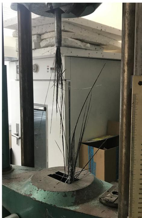
Figure 4. Specimen after failure in tension.
