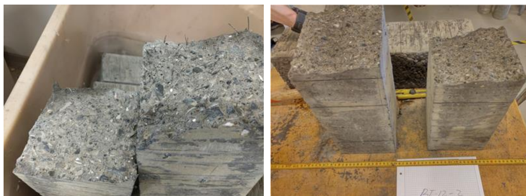
Figure 6. Reforcetech fibers are visible in the fracture but Basalttex fibers are less visible.
