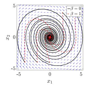
Figure 1. Van der Pol dynamics stabilized by proposed method.
