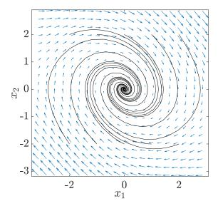
Figure 2. Pendulum dynamics stabilized by proposed method.
