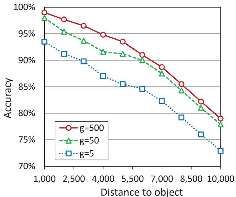
**Figure 17.** Computational experiments, detecting the distance to an object of radius  $g$  moving along the vertical trajectory.
