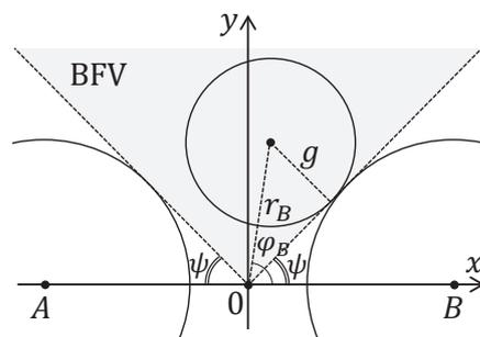
**Figure 6.** A circular feature lies entirely inside the binocular field of view if and only if  $\psi + \arcsin(g/r) \leq \varphi \leq \pi - \psi - \arcsin(g/r)$ .
