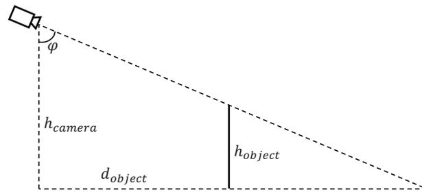
Figure 1. Simple bearing-based distance measurement model:  $d_{object} = (h_{camera} - h_{object}) \tan \varphi$ .
