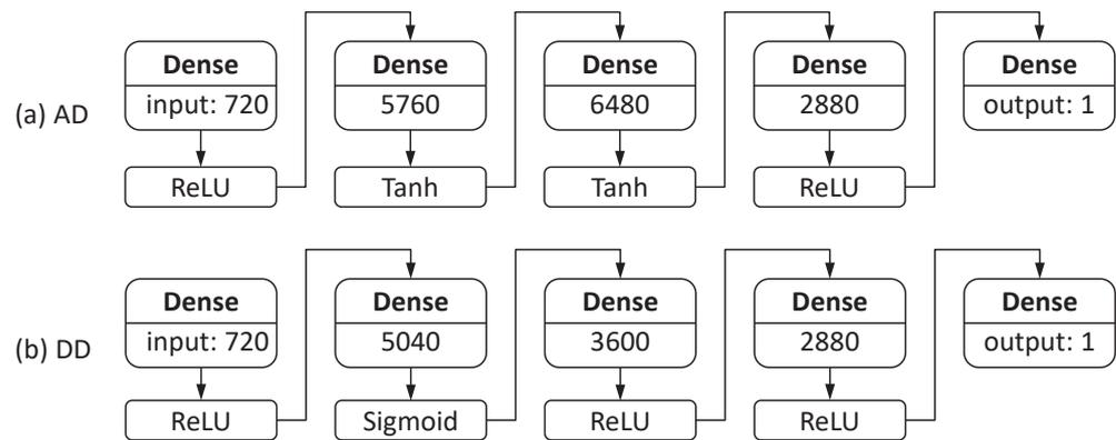
**Figure 13.** (a) AD network receives a 720-bitmap from the compound eye vision system as input data and produces the azimuth of the object. (b) DD network receives the same 720-bitmap and produces the distance to the object.
