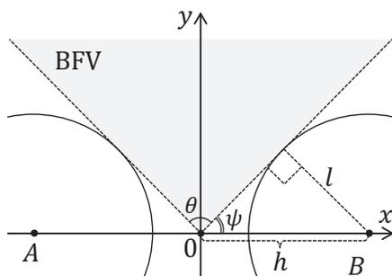
Figure 5. Binocular field of view (BFV). An object located in this area is fully visible with both compound eyes.
