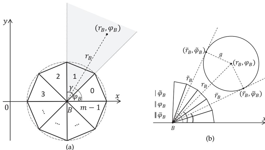
**Figure 3.** Ray tracing: (a) Point  $(r_B, \varphi_B)$  is visible for ommatidium 1. (b) Circular feature is visible for three ommatidia.
