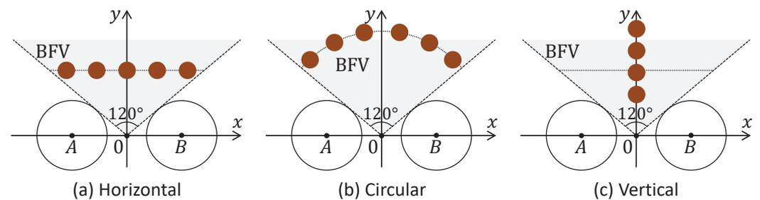
**Figure 14.** Types of trajectories for testing: (a) the object is moving along a straight line in front of the compound eye vision system; (b) the object is moving in an arc around the compound eye vision system; (c) the object is moving along a vertical line, being the central axis of the compound eye vision system.
