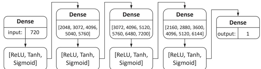
**Figure 12.** DNN hypermodel structure. Based on this hypermodel, we performed a limited random search for optimal sets of neural network hyperparameters.
