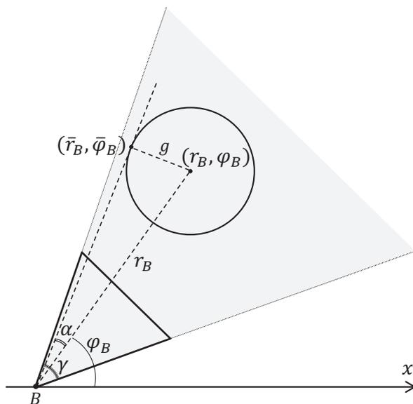
Figure 4. A circular feature is considered invisible if it is located in the field of view of only one ommatidium.
