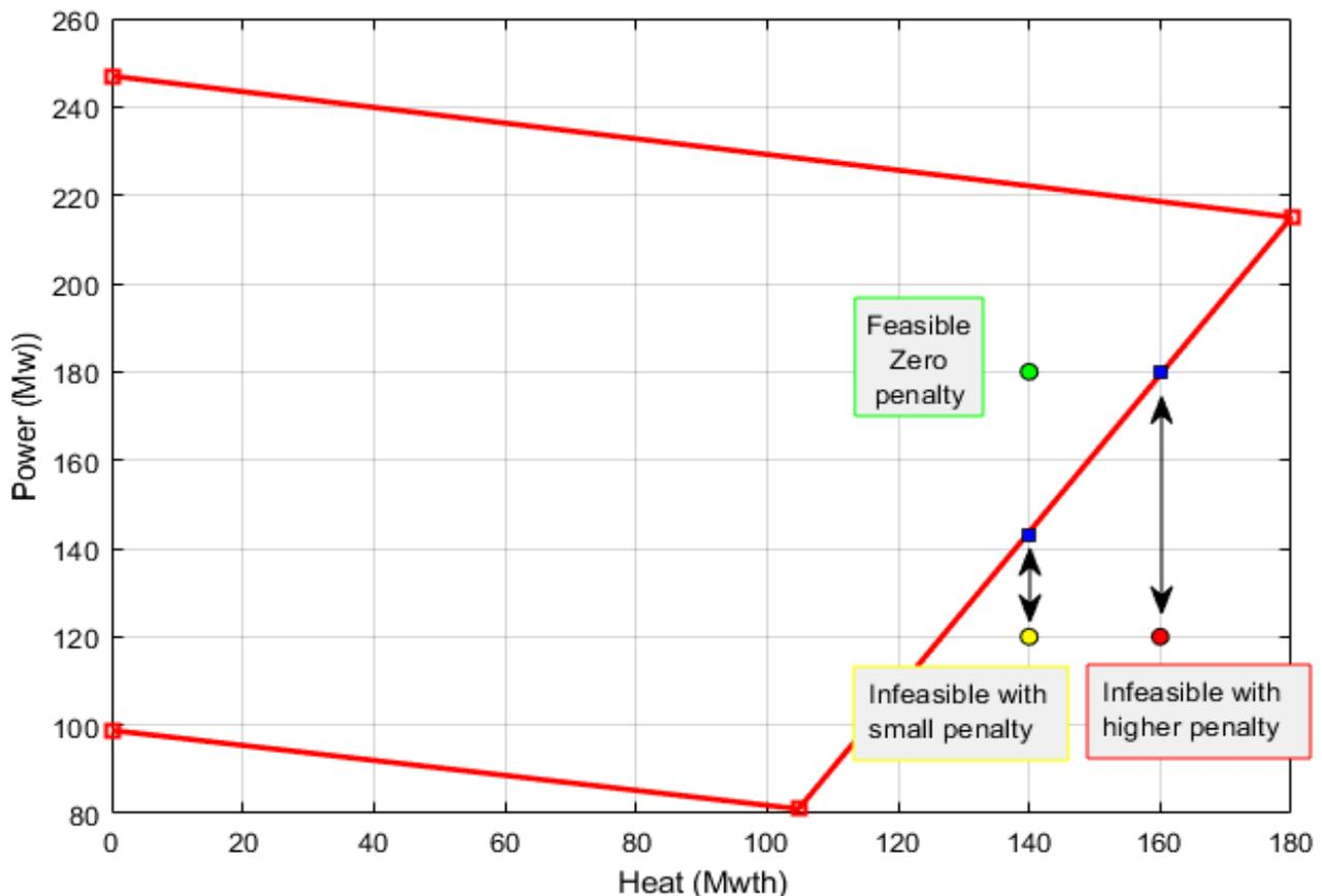
Figure 1. Permissible operating area of CHP unit.
