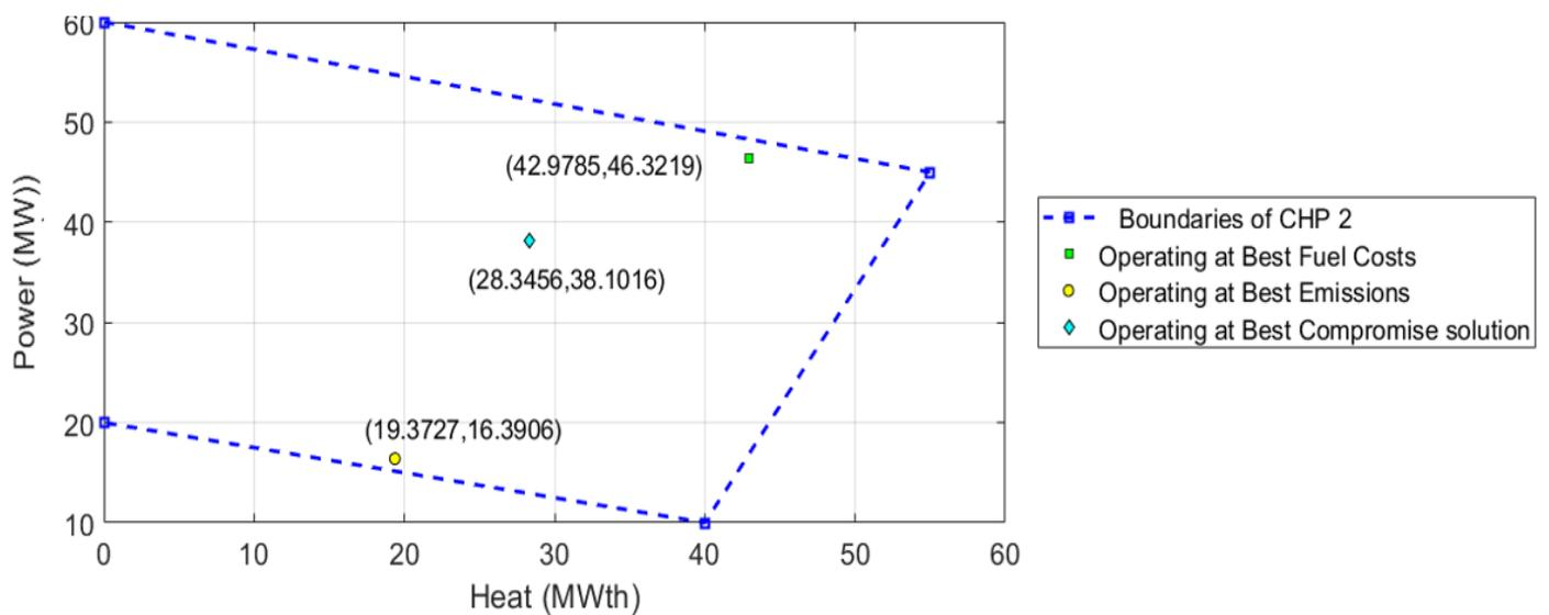
Figure 8. CHP 2 operating point versus its boundaries.
