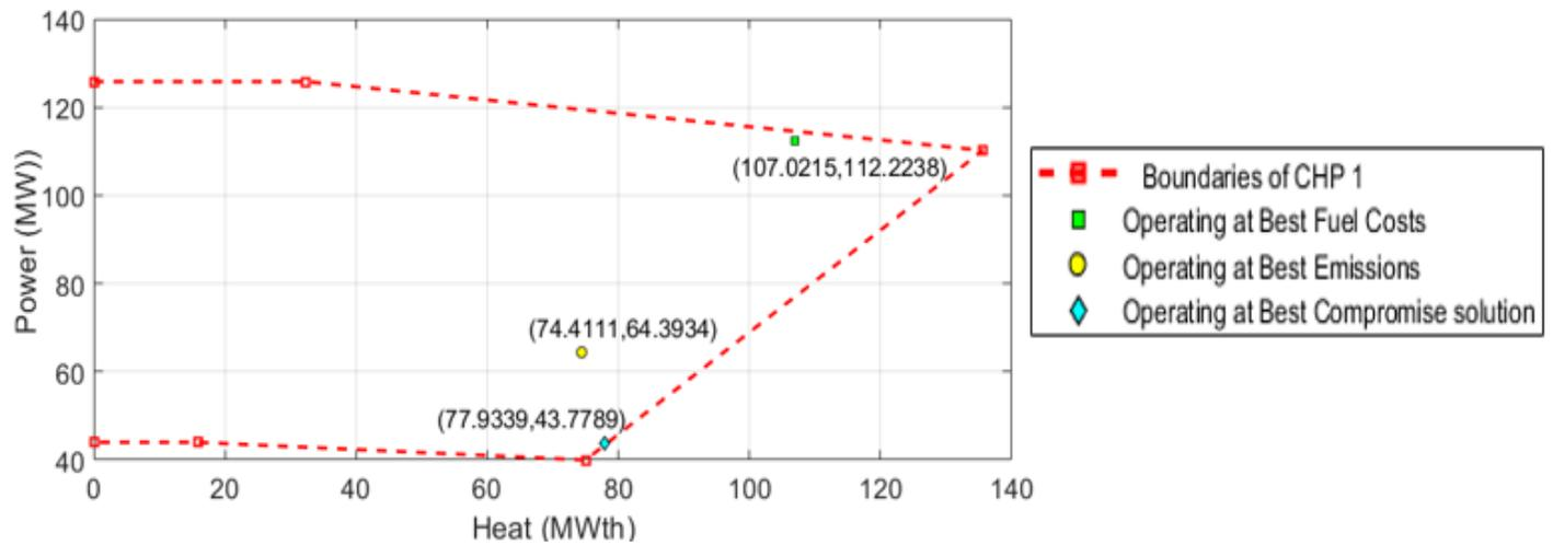
Figure 7. CHP 1 operating point versus its boundaries.
