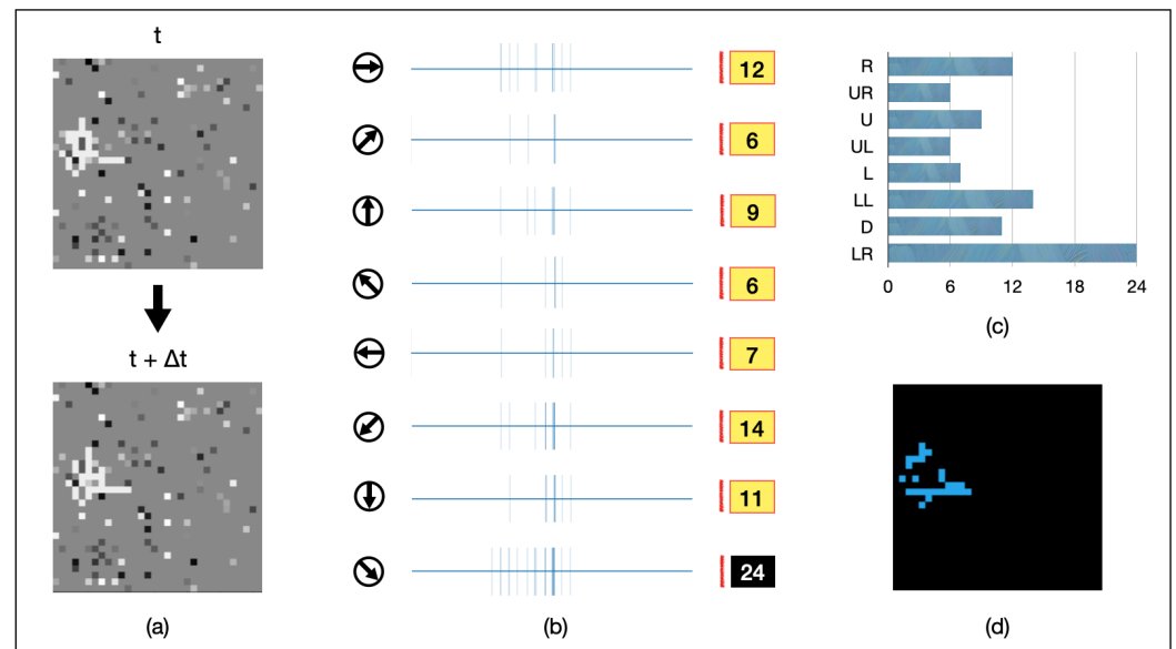
Figure 13. An AVS motion direction detection instance in static full-image noise: (a) two successive frames of a lower rightward motion of a 32-pixel object; (b) activation map of the eight LMDNs during scan; (c) LMDNs activations are counted by a bar chart; (d) activated pixels by all the LMDNs during detection process are marked by blue.
