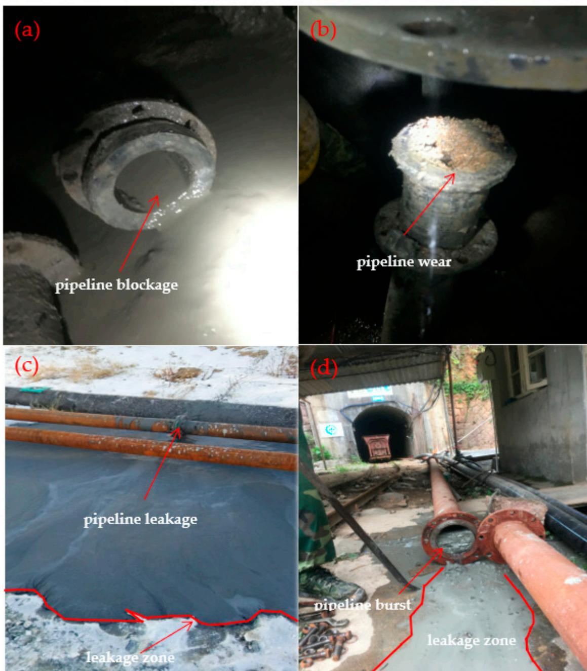
**Figure 2.** Backfilling pipeline failure photos: (a) pipeline blockages; (b) pipeline wear; (c) pipeline leakage; (d) pipeline burst.
