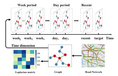
**Figure 4.** Flowchart of the data construction module. The road network is represented as a graph, and the Laplacian matrix is calculated for the graph. Instead of considering all the graphs in the time dimension, predicting a target graph is based on three types of periodic data: week-period, day-period, and recent-period.
