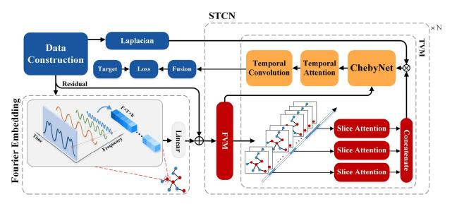
**Figure 3.** Framework of the proposed F-GCN. F-GCN contains the data construction module, Fourier Embedding module, a STCN (stackable Spatial-Temporal ChebyNet) layer including an FVM (Fine-grained Volatility Module) and a TVM (Temporal Volatility Module), and a loss function calculation module.
