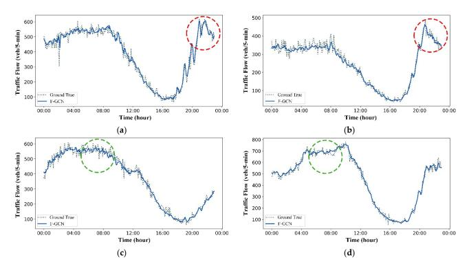
**Figure 7.** Comparison between actual traffic flow volatility (Ground True) and predicted results (F-GCN) of one-day data captured by detectors on four roads with node ID (a) 4 (b) 4 (c) 5, and (d) 9. Red and green circles represent steep and flat traffic flow fluctuations, respectively.
