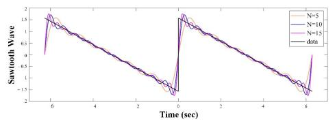
**Figure 2.** The Gibbs phenomenon in the truncated Fourier series representation of the sawtooth wave function. N represents the number of harmonics.
