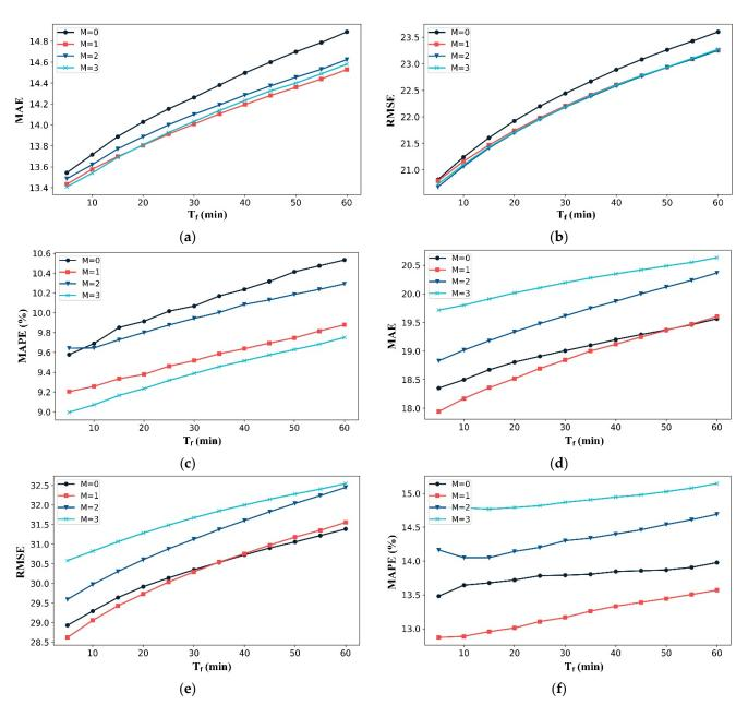
**Figure 5.** Performance of the Fourier Embedding module with a different order (M) on three indicators (MAE, RMSE, and MAPE).  $T_f$  represents the time of prediction. (**a–c**) testing on the PeMSD8 datasets, and (**d–f**) testing on the PeMSD4 datasets.
