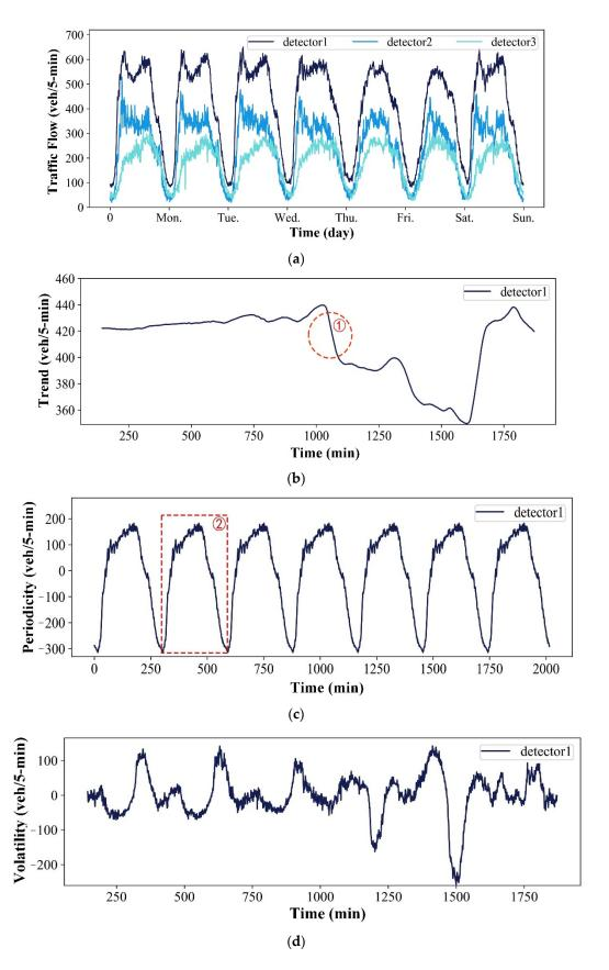
**Figure 1.** The sample detector's traffic flow data [11] in one week. (a) Original data of three detectors. (b–d) Three components (trend, periodicity, volatility) that are decomposed from the data of a sample. Trend and periodicity are marked with red dotted lines respectively.
