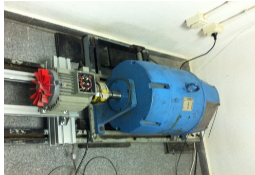
Figure 6. Induction motor coupled to the D.C. load in the experimental test bench.
