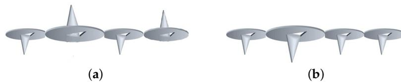
**Figure 2.** Schematic representations of surfaces: (a) up (asperities) and down (valleys) pins; (b) down pins (asperities were removed).
