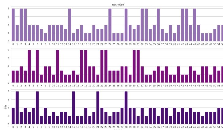
Figure A1. Quantization bit allocation of ResNet-50 following our method using the simulator. The top figure is the SCALE-Sim setup; the middle is the Eyeriss setup; the bottom is SCALE-Sim with low memory.
