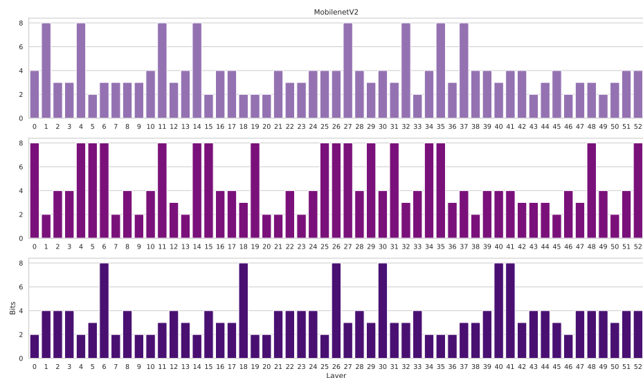
Figure 5. Quantization bit allocation of MobileNetV2 following our method using the simulator. The top figure is the SCALE-Sim setup; the middle is the Eyeriss setup; the bottom is SCALE-Sim with low memory. Depthwise convolutions have a higher feature map and, thus, higher memory footprint, and we can see that Algorithm 2 allocates fewer bits when the system memory is low, i.e., the model is memory-bounded. Models with higher memory allocate the bits differently due to the locality of the boundary (memory or computational) by the layer. This figure does not include the first and last layers, which we quantize to 8 bits.
