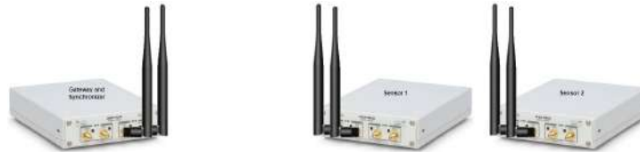
Figure 19. Two-sensor and one gateway experiment setup using NI-B210 SDRs.
