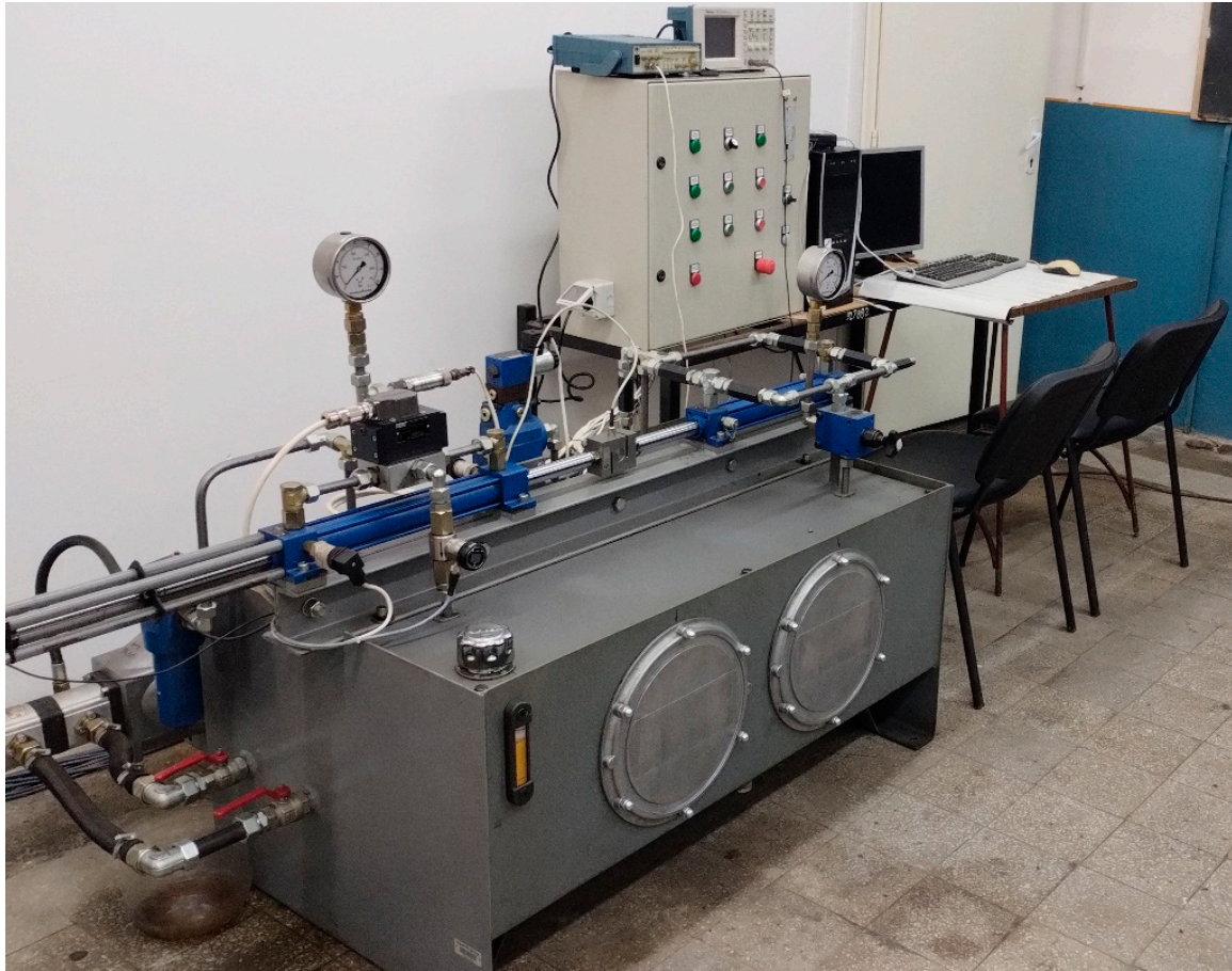
Figure 1. The test rig emulating the wind turbine blade pitching system.
