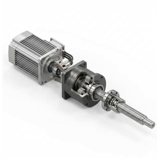
Figure 2. Canonical primary flight control actuator (PFCA) architecture: The coupled drivetrain comprises a high-speed AC motor, planetary gearbox (AISI 9310 steel), and ball screw transmission (52100 steel). Gearbox fatigue-induced vibration propagates to the ball screw, accelerating fretting wear—the coupling mechanism central to this study.
