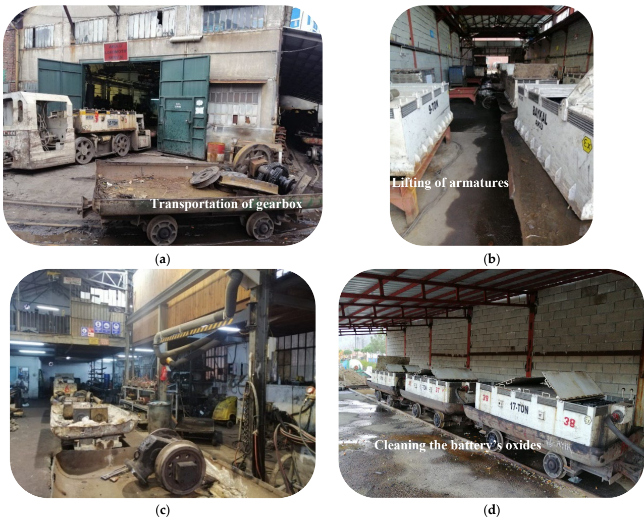
Figure 1. View of the battery locomotive service and charging unit at Karadon Hard Coal Company: (a) entrance of the maintenance workshop; (b) 9-ton batteries at the charging points; (c) interior of the maintenance workshop; (d) cleaning the battery oxides.
