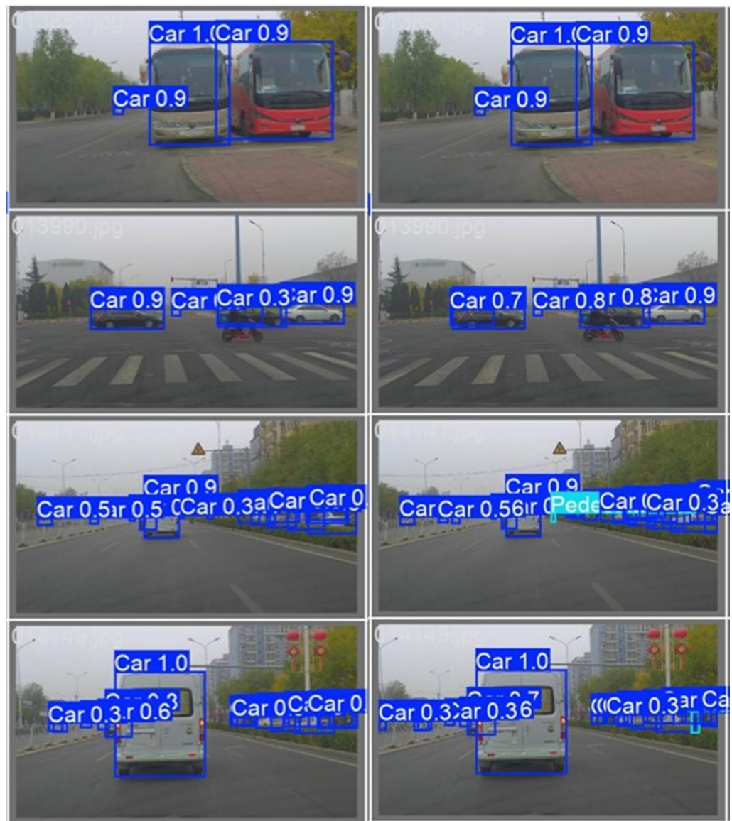
Figure 5. Qualitative detection comparison on the DAIR-V2X vehicle-side dataset. In each paired example, the left panel shows the YOLOv8n baseline detections and the right panel shows the YOLOv8n-FEL detections. KITTI-trained models are directly evaluated without DAIR-V2X fine-tuning.
