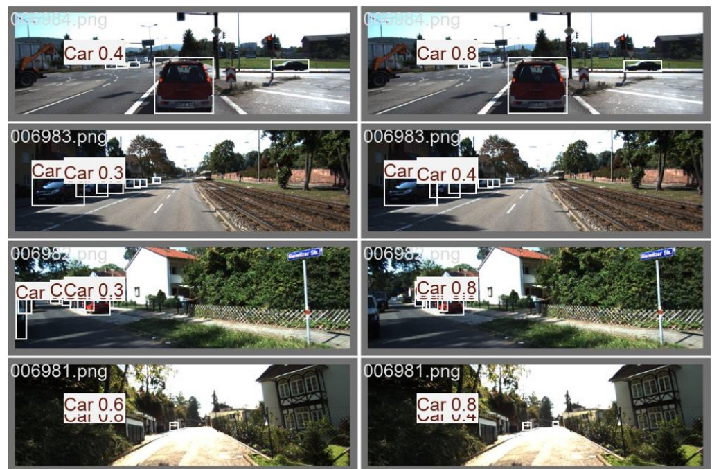
Figure 3. Qualitative detection examples on the KITTI validation set. Each pair compares YOLOv8n baseline detections (left) with YOLOv8n-FEL detections (right) under identical input conditions. The examples are illustrative and should be interpreted together with the quantitative AP results.
