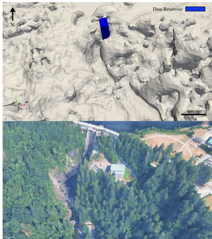
Figure 3. Computational domain of the Cleveland Dam and surrounding Capilano River valley, with comparison to real-world topography from Google Earth Pro [57].
