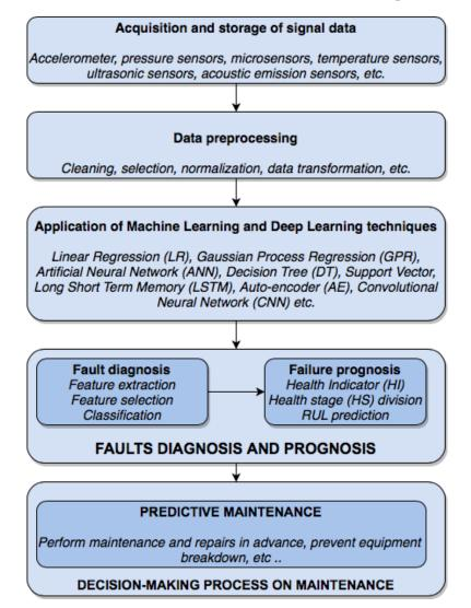
Figure 3. Schematic representation of predictive maintenance.
